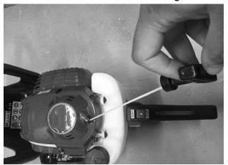
In all the cases, after starting, put the lever of the choke on.
